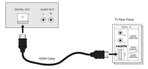
1) Connect the HDMI Cable from the DIGITAL OUT on the back of your DTV or HDMI device, to the DIGITAL-IN on the back of your television.
